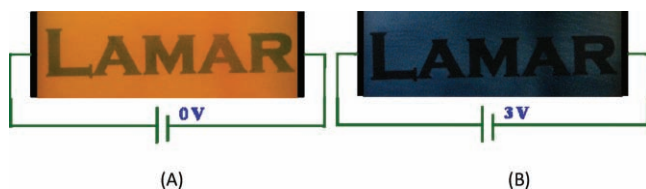
Figure 8. The color change of the PBZT thin film before (A) and after (B) applying a voltage.
